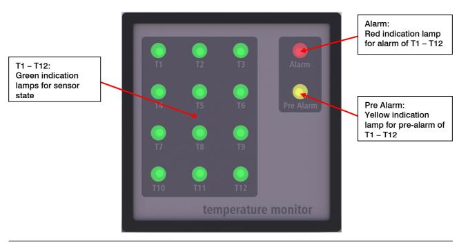
The indication lamps (green) of the sensors T1 – T12 can show the following conditions:
