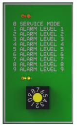
**Position 0** activates the service mode. If selected, all connected CS sensors are working in analog mode and the current object temperature can be checked with a volt meter on each separate service point **[SP]**.
