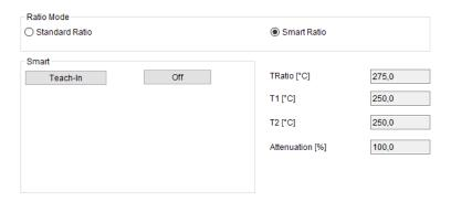
A requirement for the measurement is that the object temperature must be known.
