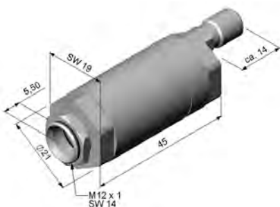
Standard air purge collar, may be combined with mounting bracket
