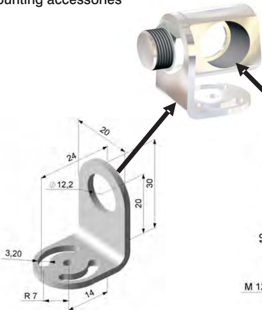
Mounting bracket, adjustable in one axis
