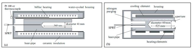
Schematic layout of heat pipes used at the PTB: sodium and caesium heat pipes (a) / water and ammonia heat pipes (b) [3]
